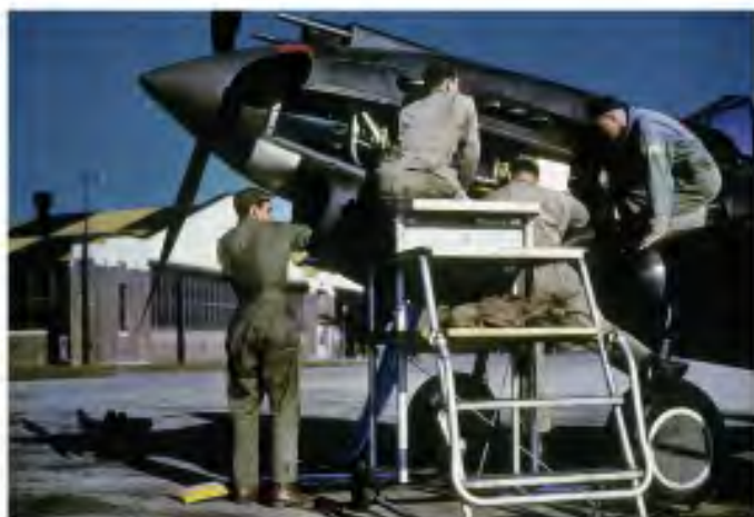
The Curtiss P-40-CJ was powered by the Allison V-1710-33 engine, and in this photograph, Army Air Corps mechanics are servicing one of these engines and its accessories. Above the cooling section, the intake for the first 30-caliber machine gun. Stan-Piet collection
