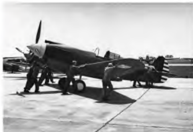
Ground crewmen push a P-40-CJ of the 49th Pursuit Group into position on a hand-paved strip homebase at Langley Field, Virginia. This aircraft was modified number 842 and had a 100-hp Allison V-1710-33 engine. The 30-caliber machine gun intake is visible above the landing. Timeline Museum of the United States Air Force
